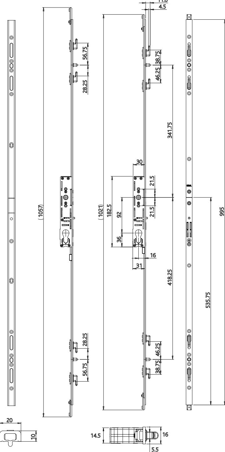
Diagram illustrates product in locked position. All dimensions are in mm and are nominal. ERA reserves the right to change specification without notice. It is the responsibility of the door manufacturer to ensure that the finished product meets any required safety and performance specification without notice.
