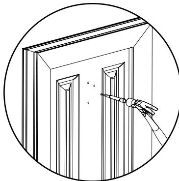
4 If fitting to PVCu profile, use a 2mm drill bit to pre-drill the fixing holes ensuring the drill bit pierces the steel re-inforcement. If fitting to timber drill to a maximum depth of 15mm.
