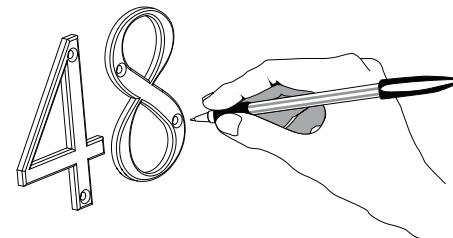
3 Remove the numerals. If available always use a drill punch to mark drilling positions using the pencil marks as a guide. The indent made by the point will ensure the drill does not slip.
