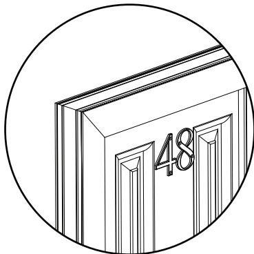
2 With the numerals correctly located mark the fixing holes with a pen or pencil.
